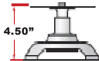
1969 1/2 and Later Measures 4.50'' From Pulley Flange To Mounting Surface
