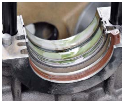
For final assembly, Jeff prefers to use 60W motor oil for pre-lube and uses the Viton rear main seal from JPW. He staggered the block and cap halves, as shown, to help prevent leaks.
