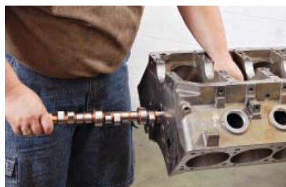
During preassembly, Jeff installed the Comp hydraulic roller cam to ensure that it rotated freely in its bearings.
