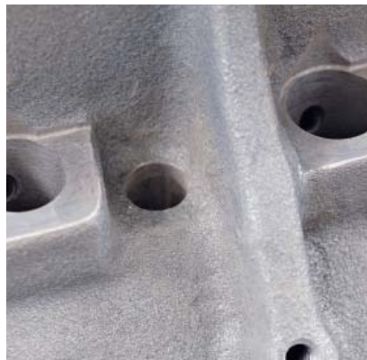
Jeff drilled oil drain holes in the lifter valley, as this block comes prepped to run a dry sump oiling system. The Comp Cams hydraulic roller lifters will drop in with no modifications needed to the block.
