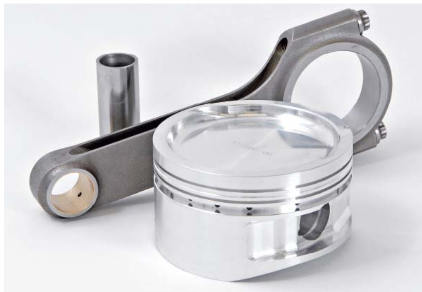
Full-floating .990-inch Ferrea pins connect the custom Ross forged pistons to the Scat 6.700-inch high-tensile 4340 forged H-beam rods featuring 2.20-inch diameter big end to fit the big-block Chevy-sized crank journal. For this O-deck engine, the compression ratio of 7.96:1 will result from the 49cc dish in the pistons, 90cc chamber E-heads, and the volume of the head gasket.
