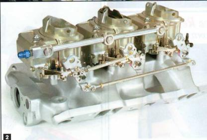
1 Pontiac's original Tri-Power setup is an icon—but not necessarily the best or most cost-effective way to make horsepower. Besides being expensive, they generally give up 35-50 horses over a well-tuned single four-barrel induction system.
