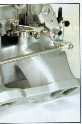
could scarcely believe his eyes given his experience with other 3x2 induction systems on this same engine package. Looking over the numbers, the Demon 6 The front and rear carbs have their idle-discharged circuits linked to the transfer slots and their idle mixture and idle speed adjustment screws preset (no synchronization required). The central carb also has a provision for constant vacuum and ported vacuum. Also, the rear carburetor is provided with a PCV port.
