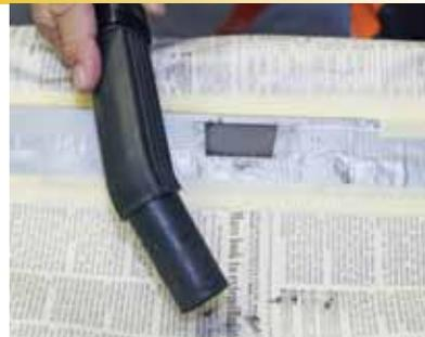
**10** Once the cement was fully cured, it was checked for flatness using a straight edge—it was perfectly flat. Any high spots can be knocked down with sandpaper or a file if needed. A wet/dry vacuum was then employed to suck up all traces of dirt and debris before removing the tape and newspaper. Several passes were made to ensure that absolutely nothing would enter the engine. Even the slightest amount of grit can create significant internal damage.
