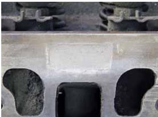
**11** Removing the masks and tape revealed that the cement-filled opening was in fact completely flush with the intake flange. If a depression exists, the only real recourse is to chip the cement away with a hammer and screwdriver and start over again. (In either instance, be sure to carefully mask accordingly to keep contaminants out of the engine.) ◀
