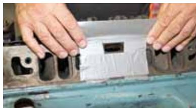
**7** After removing the intake manifold and existing gasket, the intake flange was wiped clean of grease and oil using a lint-free cloth and brake cleaner. Then quality duct tape was used to seal off any opening on the flange that might allow the cement or dust/debris to enter the intake ports.
