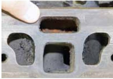
**2** Beginning in '72, Pontiac added this hole above the exhaust crossover. Said to keep oil flowing under the valve cover isolated from exhaust heat, it's completely separate from the crossover and does not connect to any other port or passage.
