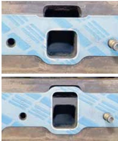
**3** The exhaust crossover of the corresponding '72-later intake manifold gasket is accordingly sized to accommodate the blind hole (top). Earlier gaskets use a larger exhaust crossover opening; that can result in a significant exhaust leak at the flange when using any Pontiac intake manifold (bottom).
