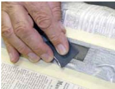
**9** A putty knife was used to carefully scrape away the excess cement, and lightly wetted 400-grit sandpaper smoothed the surface. It's important that the cement is flush with the intake flange, as any recess can prevent the gasket from properly sealing. The identical procedure was performed on the opposite cylinder head and both were allowed to dry overnight.
