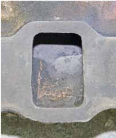
**5** Through '71, the intake manifold's right-hand exhaust cross-over passage is nearly double the size of the lefthand port. It was likely intended to reduce the amount of material located directly under the choke stove, providing optimal warm-up time. Exhaust leaks are common when combining a manifold of this vintage with later cylinder heads.
